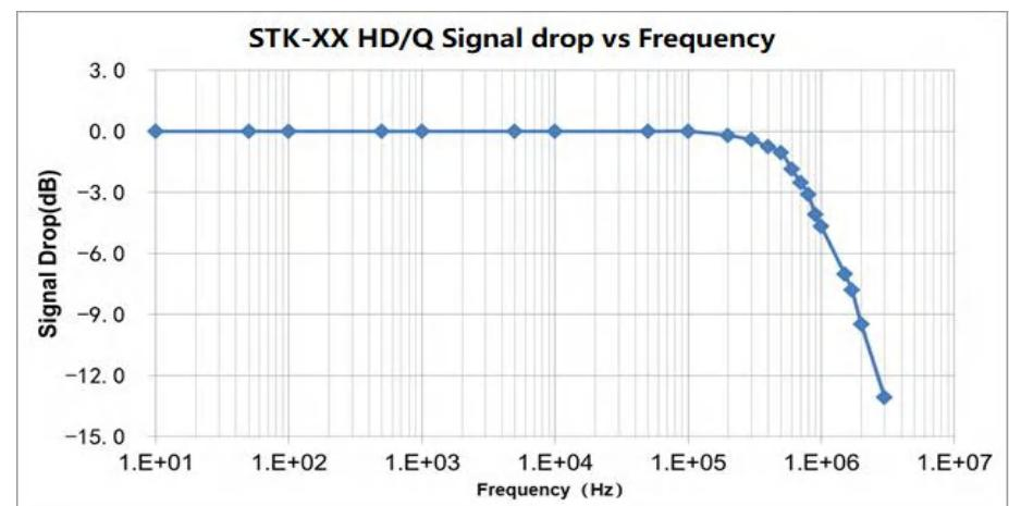
The frequency bandwidth of STK-HD/Q series current sensor. The bandwidth of current sensor is DC ~ 400 kHz (-3dB).
